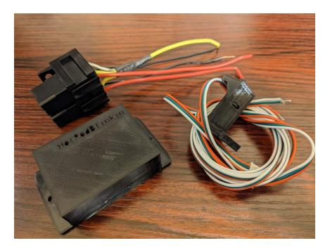
HotRodBlinkn' fills a need for us HotRod and Custom Vehicle enthusiasts. In particular, the Factory Five Roadster that I built which inspired the creation of this module. So often these builds use a simple generic steering column, with no provided mechanism to have a self-canceling turn signal.
